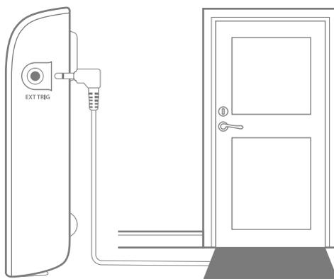
2. Connect the contact mat to the ext. trig. outlet on the Visit transmitter. Place the contact mat within reach from the transmitter and so that the cable can be fitted securely.
