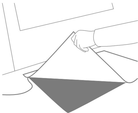
1. Place the contact mat on a flat, smooth surface and mount the cables to the wall or baseboard. Cover the contact mat with a carpet or entrance mat to protect it from daily wear and to avoid slip hazards.
