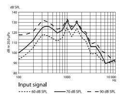
Output signal with BE9125, Stetoclips
