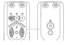
The sound from the Transmitter Unit is mixed with the sound from the internal microphone. You can adjust the balance between the Receiver Unit and the Transmitter Unit's microphone by holding down the MIC button (5) at the same time as setting the balance using the (11) or buttons (12).
