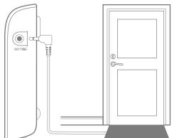
2. Connect the contact mat to the ext. trig. outlet on the Visit transmitter.
